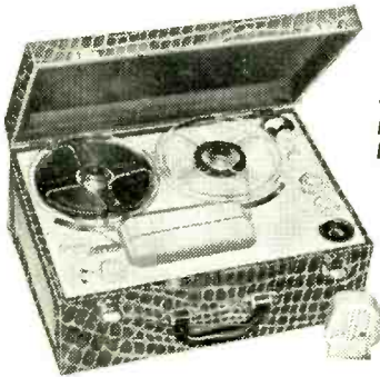
Four-valve portable embodying T.C.C. printed-circuit element.
