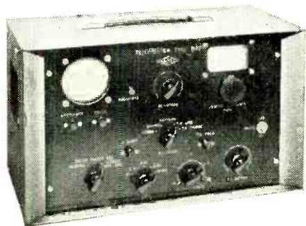
Airmec "Televet" television receiver alignment and test equipment.
