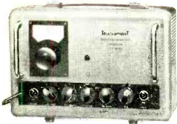
Telegroup 2-band television pattern generator, Model WG44.
